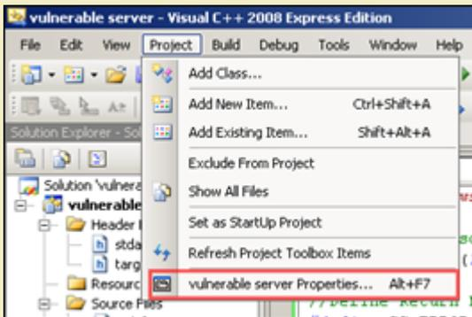
Go to C/C++, Code Generation, and set "Buffer Security Check" to No
